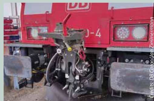
Hybrid DAK an einer Alstom Traxx 2-Lokomotive (BR 185) der DB Cargo. Hybrid DAC on an Alstom Traxx 2 locomotive (BR 185) of DB Cargo.
