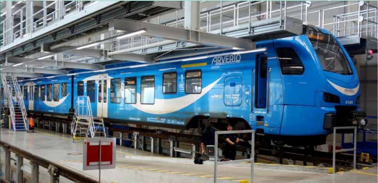
Access to the train from above, below, and the side: a modern, ergonomic workstation at EUCO Rail in Langweid. Credits (6): Hermann Schmidtendorf
