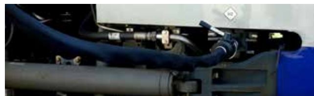
Here, a Mireo Plus H is being refueled with hydrogen directly from the refueling system.
