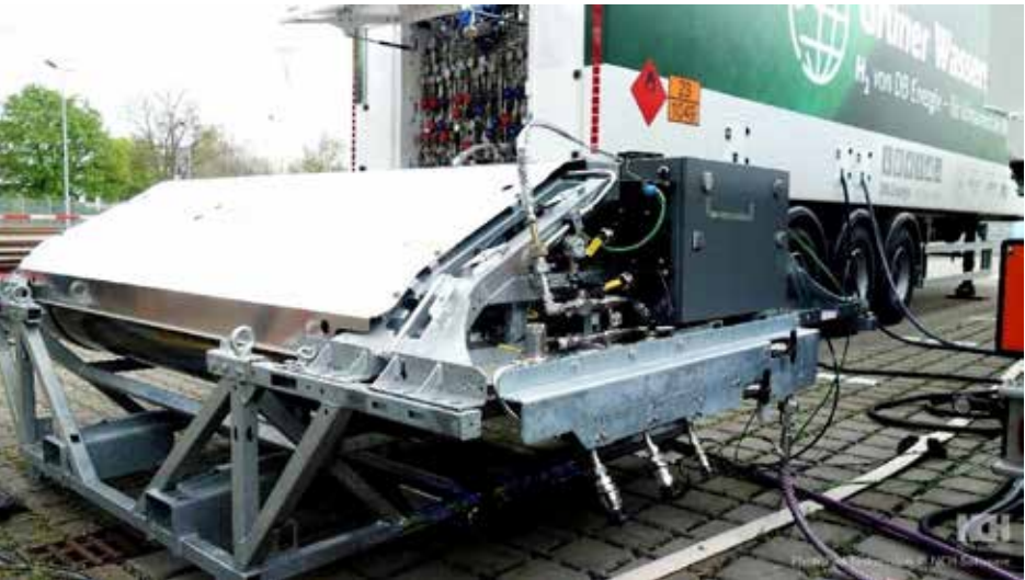
A Mireo Plus H is being refueled in southern Germany from this mobile DB Energie trailer.
