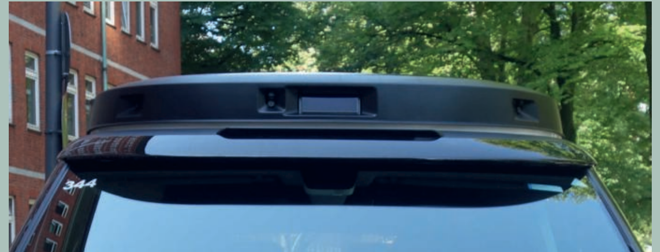
Cameras and sensors on the roof of the vehicle constantly monitor and control its progress.
