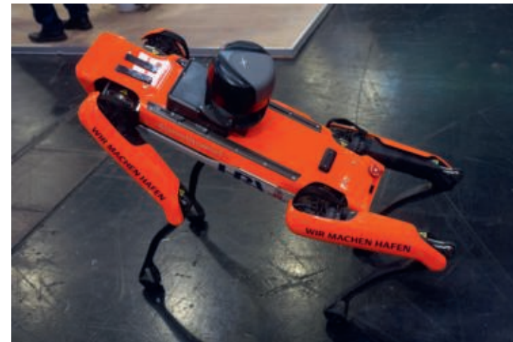
Agile: The SPOT robot for inspection work.
