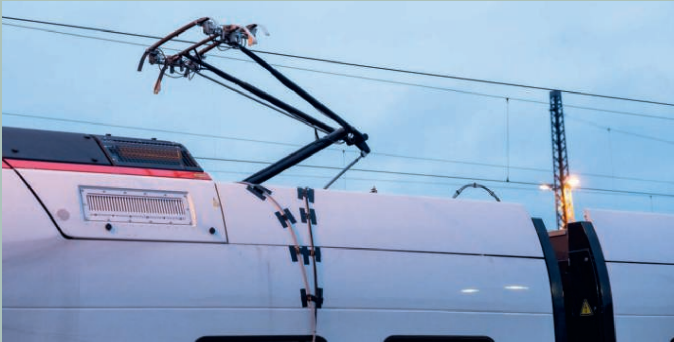
A pantograph of the KISS double-decker carriage during testing
