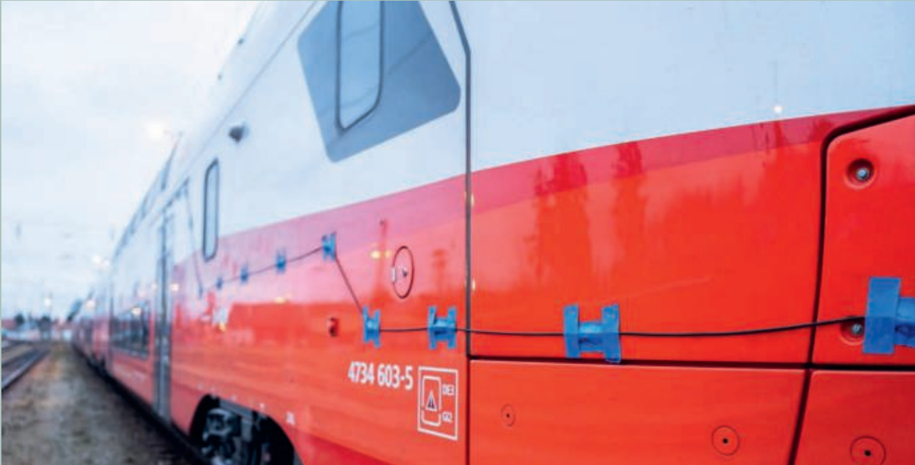
The side wall of the tested double-decker carriage with attached sensors.
