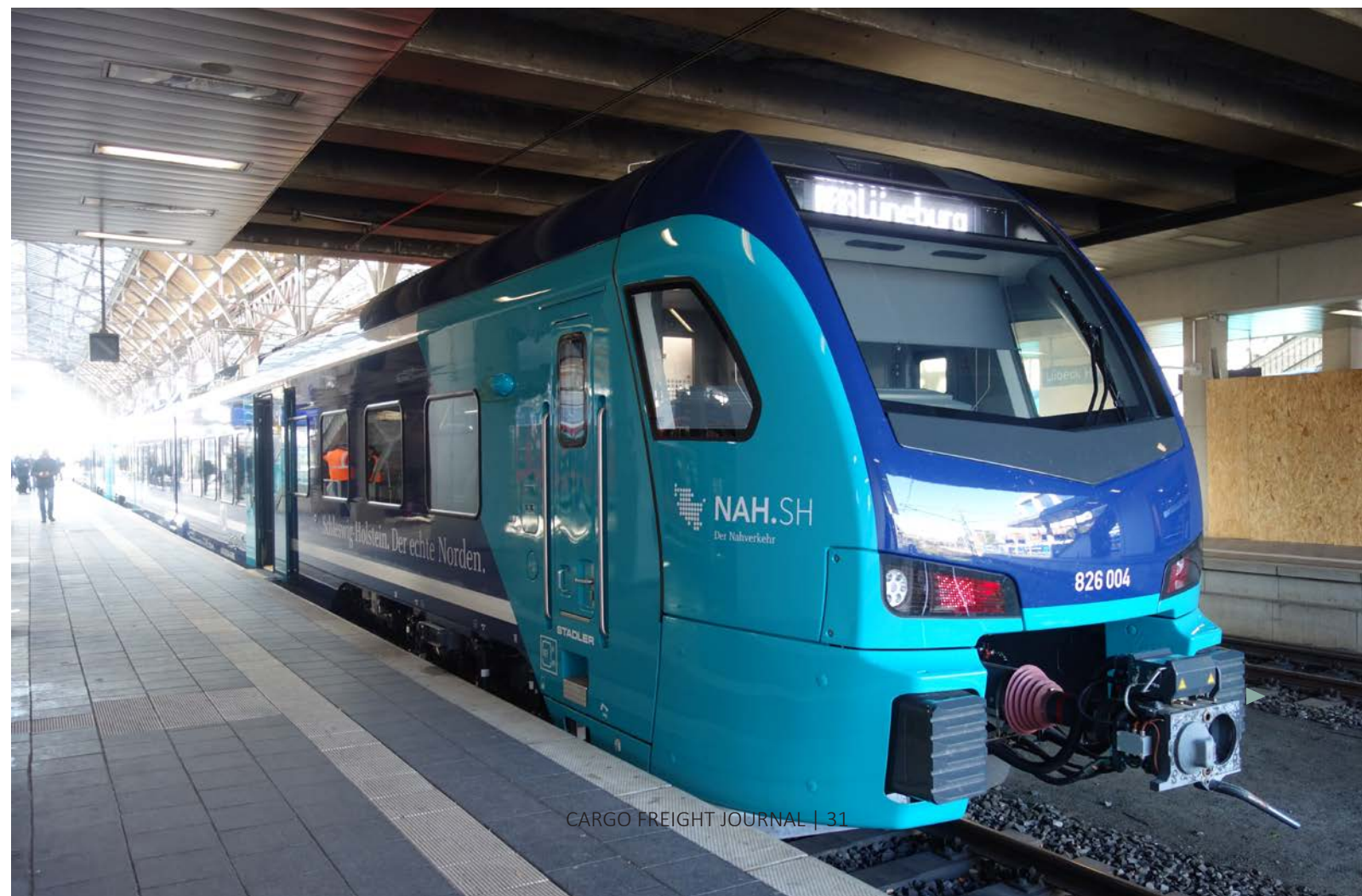
A battery FLIRT at Lübeck main station.
