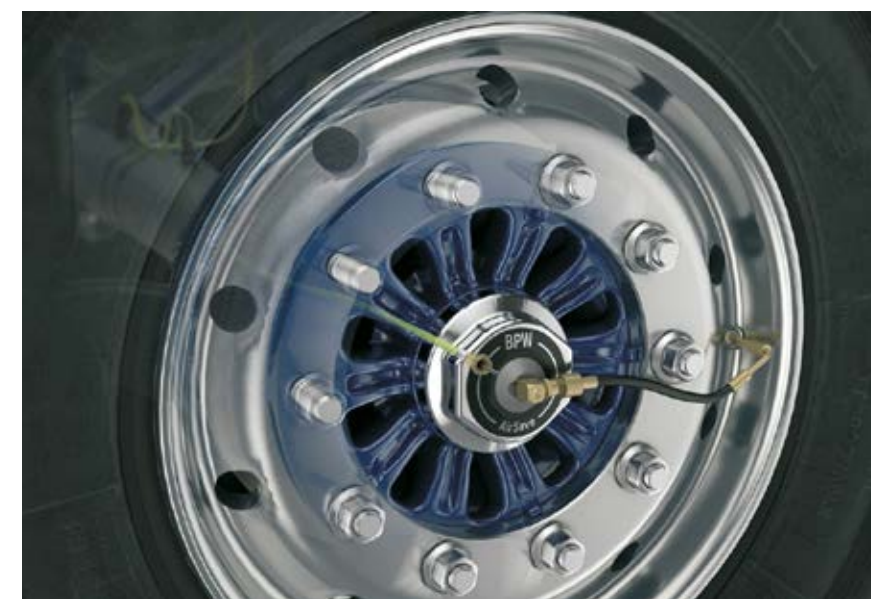
A small tube between the wheel hub and tire shows that this vehicle always runs with optimal tire pressure thanks to the AirSave system.
