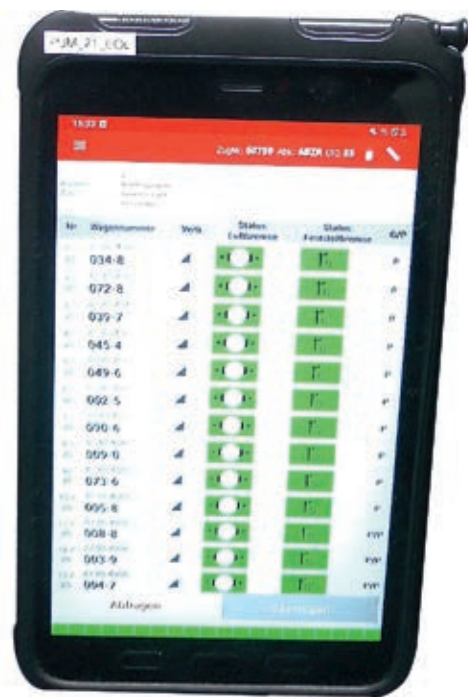
The results of an automatic brake test can be read for the entire train in just a few minutes on a handheld.
