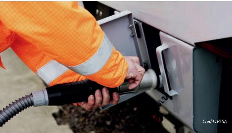
An unspectacular process – refueling the PESA locomotive with hydrogen, here on the Polish test site in Żmigród.
