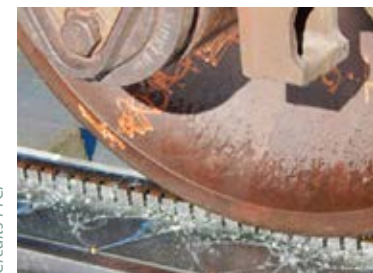
A wheel with a crack on the Tycho detection facility.
